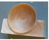
Ed started by explaining that a wood face plate was needed to temporarily mount the piece in the different orientations. He made his face plates out
