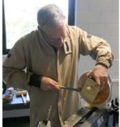
the face plate using the double sided tape. The tail stock was pulled up to hold the block in place and a bead of hot glue was added around the block to further secure it to the face plate. Ed let the glue cool before proceeding
