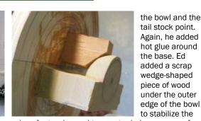
piece for turning and to counter-balance some of the off center weight in the piece being turned. He added tape and glue to hold the scrap to hold it in place while turning.
