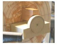
Ed attached double sided tape to the bottom of the piece and carefully centered the piece on the face plate using the center mark of
