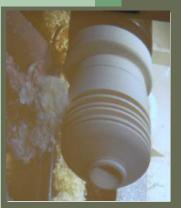
and of uniform thickness. The slot was the width of the parting tool that was kept very sharp from repeated use of the grinder or a hand held diamond hone. Ed kept the speed up around 1,500 rpm's to get a clean cut. When all the parting cuts were a uniform depth and all cuts
