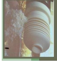
parting it off would leave about 1/2" of solid wood. The vase was then parted off from the waste block in the chuck with a slight undercut to leave a slightly concave rim on the base and a slight rounding of the outer edge of the base.
