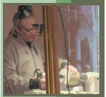
as you can hollow it out. Ed used white ash about 4-5" in diameter and 1012" in length. The piece was mounted between centers on the pith and turned round using a roughing gouge. All the bark was removed and the piece rounded into a cylinder. A tenon was added to one end.
