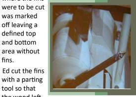
was perpendicular to the central axis of the piece and of uniform depth. The width of the wood fin was about 1/8" to 3/16" wide
